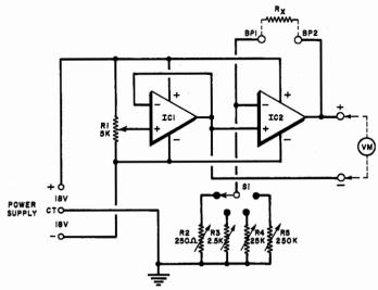
Linear scale ohmmeter uses two intergrated circuits. When the circuit is properly balanced (via range switch and potentiometers), the meter reading is proportional to the unknown resistor.
